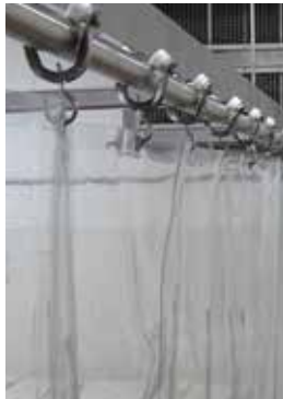
Open trolley design to prevent bacteria from forming.
