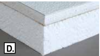
D. 1-1/2" EPS Foam is laminated to 1/2" fire & moisture-resistant gypsum and FiberLite FRP one side only. 2' x 4'.
