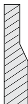
Cross section of Brute belly patch . . . patch is cured directly into fabric.
