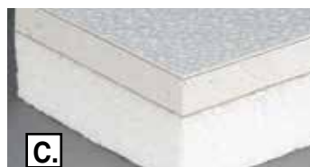
C. 1" EPS Foam is laminated to 1/2" fire & moisture-resistant gypsum and FiberLite FRP one side only. 2' x 4'.
