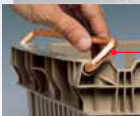
Two 3/8" zinc-plated steel wire bails swing down to allow nesting and swing up for stacking.
